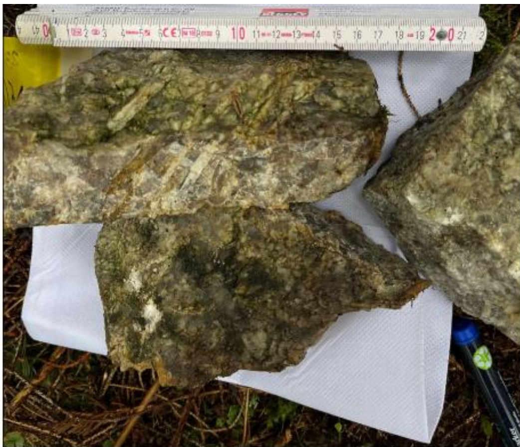
Figure 5. Photo of sample 230717 from Pusterwald area (see Table 1 above for lithium result); note the large grained spodumene crystals
