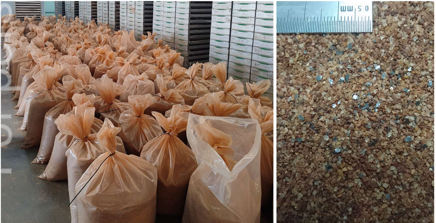
Figures 1 & 2: LHS: Four tonne graphite pre-concentrate sample produced at the Company's Lilongwe laboratory RHS: Close-up of the pre-concentrate showing the coarse, clean graphite flakes
