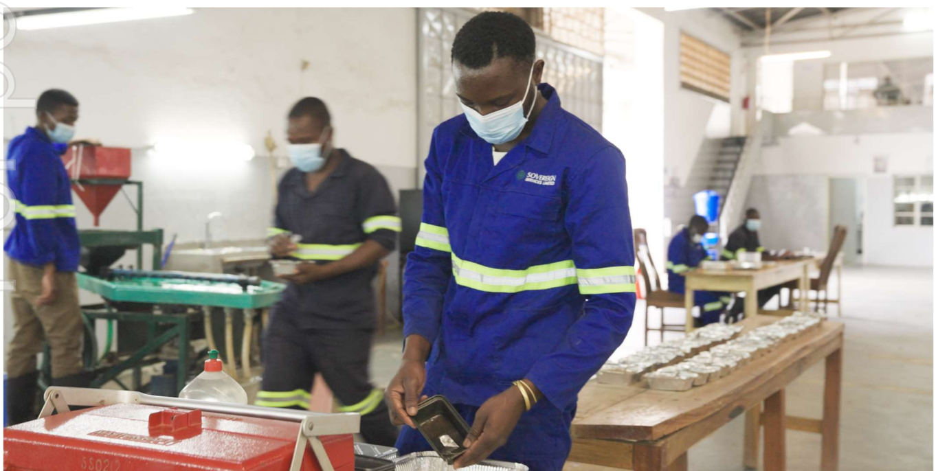
Figure 4: Logging and weighing sample at Sovereign's bespoke Malawi laboratory
