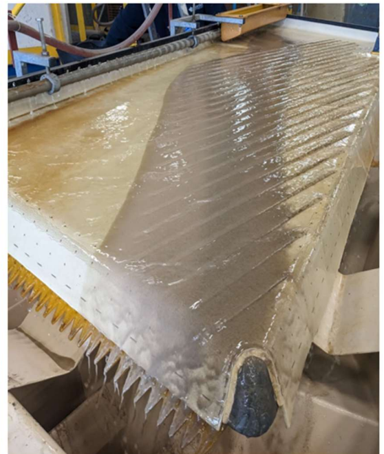
Figures 5 & 6: LHS: Kwatani shaking screens prepared for despatch to Malawi. RHS: An example of the Holman-Wilfley 2000 Series shaking table that has been ordered and is currently under fabrication
