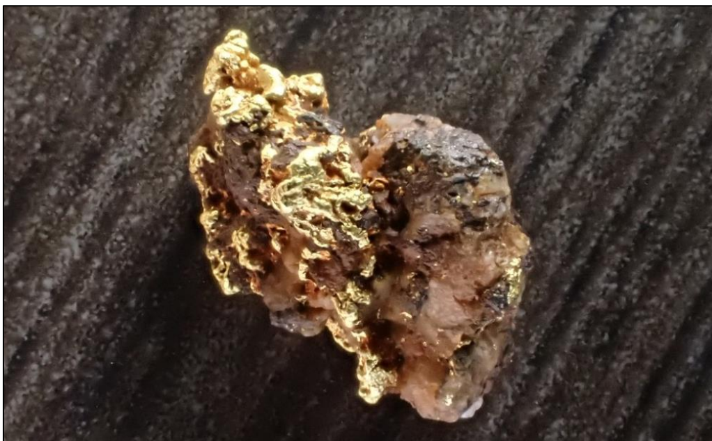
Figure 8 Angular gold from Guyer with iron oxides (after sulphides) in a quartz vein fragment (from ASX release dated 21 November 2022).
