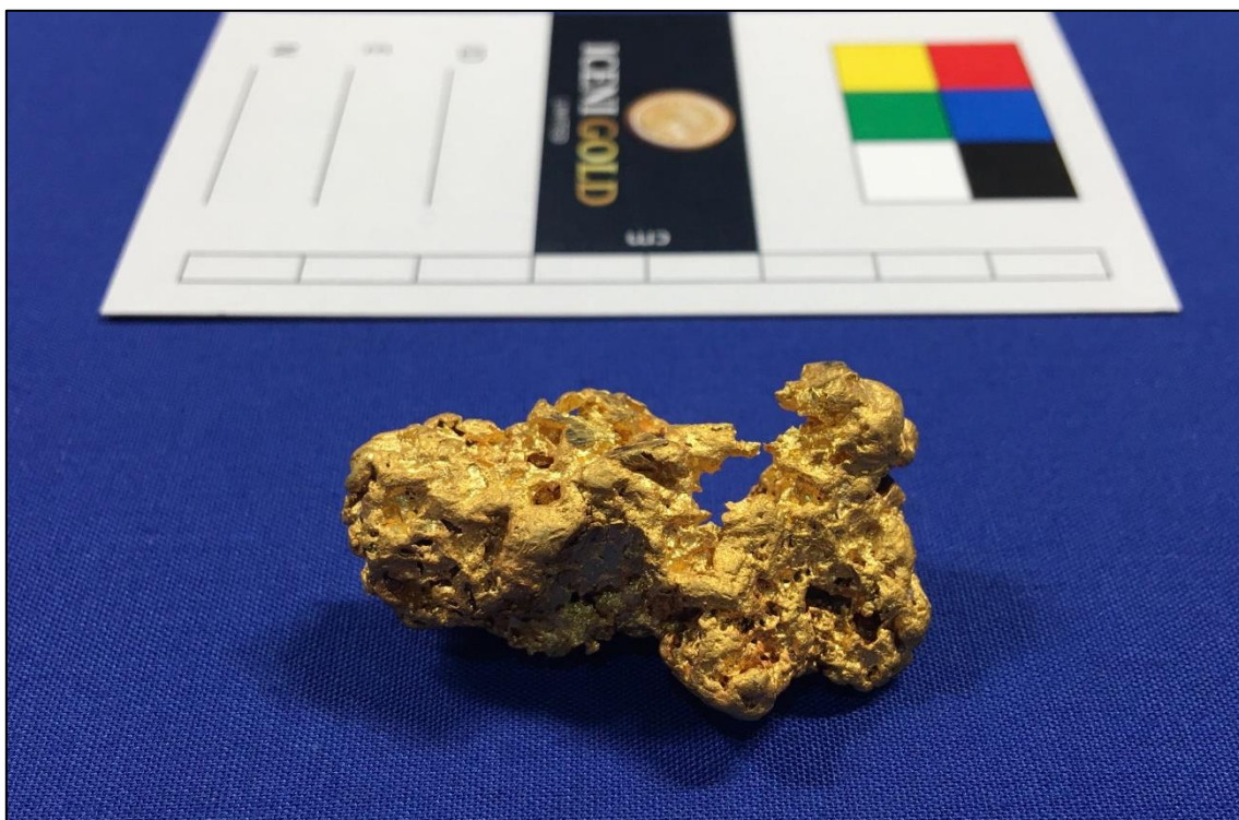
Figure 2: Nugget* GY-1 after cleaning. The nugget has a gold fineness of 99.1% (measured by pXRF).
