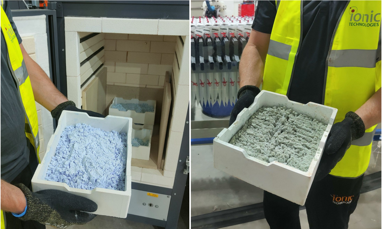
Figure 1: First separated magnet rare earth oxides produced from Ionic Technologies’ Belfast Recycling Demonstration Plant, showing >99.5% Neodymium oxide ( \text{Nd}_2\text{O}_3 ) on left, and Didymium oxide ( \text{NdPr} oxide) on right.
