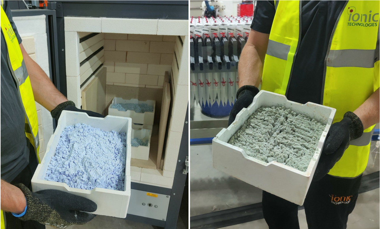
Figure 1: First separated magnet rare earth oxides produced from Ionic Technologies’ Belfast Recycling Demonstration Plant, showing >99.5% Neodymium oxide (Nd 2 O 3 ) on left, and Didymium oxide (NdPr oxide) on right.
