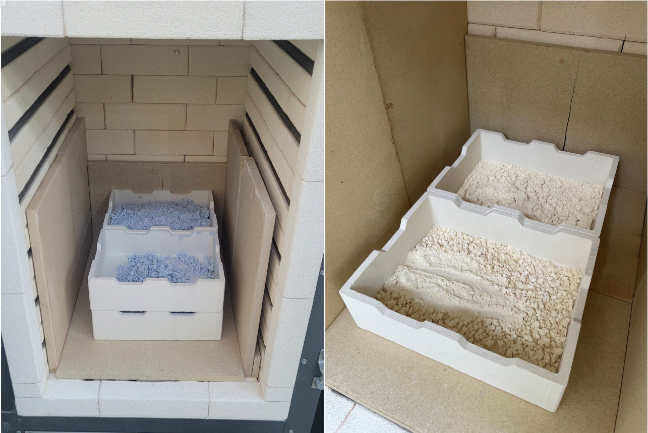
Figure 2: Calcination of \text{Nd}_2\text{O}_3 on left, and \text{Dy}_2\text{O}_3 oxide on right.
