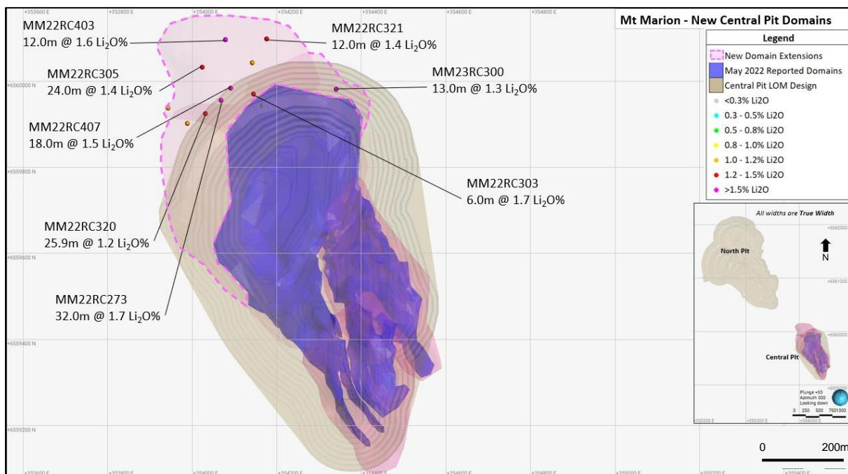
Figure 6: Central Pit resource extension (plan view)
