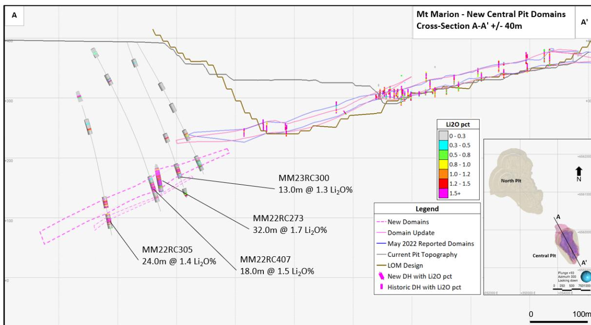
Figure 7: Central Pit resource extension (long section)
