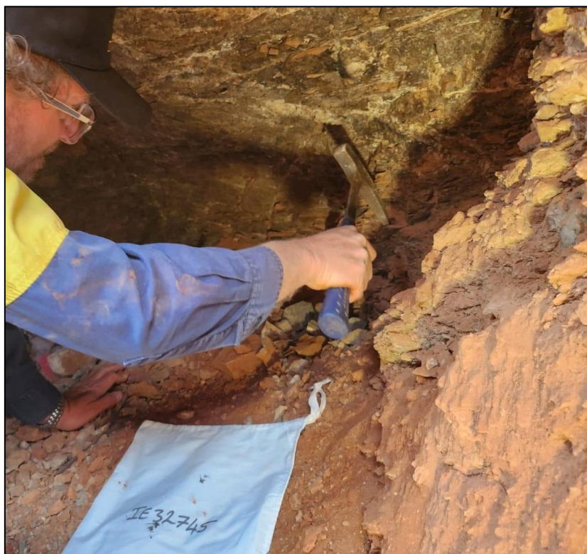
Figure 3 Sampling mineralised sediment exposed within the workings. Gold and sulphide bearing quartz veins have been observed, associated with the sediment-andesite contact.
