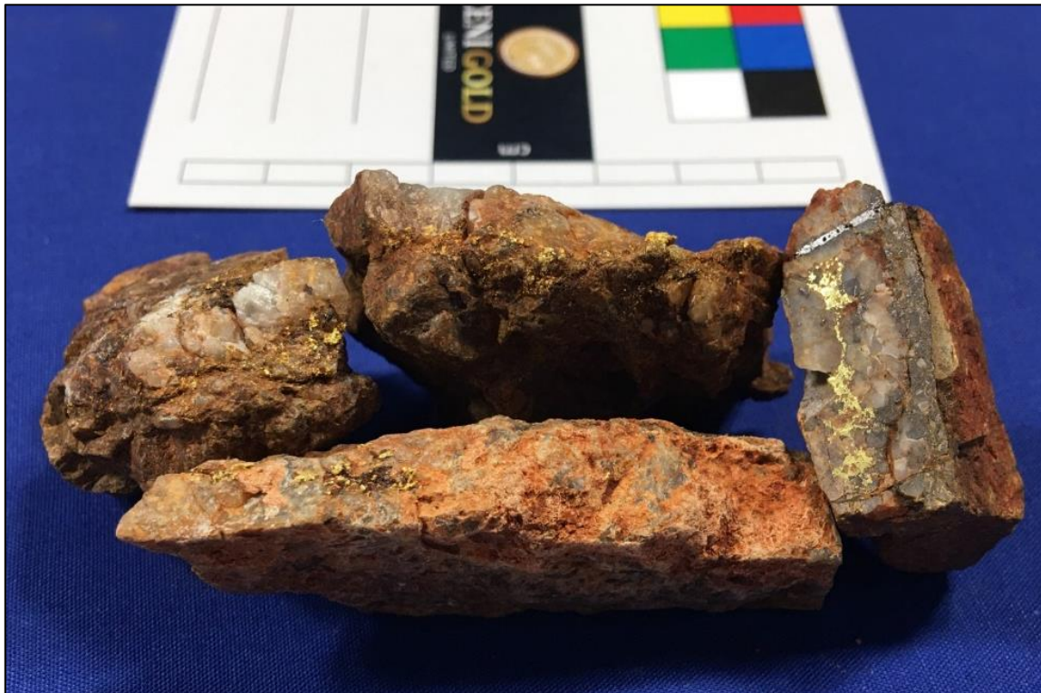
Figure 7 Specimen EV-4, gold taken from outcrop within the Christmas Gift anomaly (14UF010B). The peak assay was 18,207g/t Au (previously reported in ASX release dated 8 June 2023).
