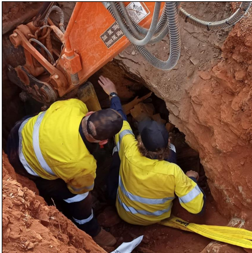
Figure 2 Observing geometry of the mineralisation visible within the historic workings. Veining was measured to strike between 320° to 340°.
