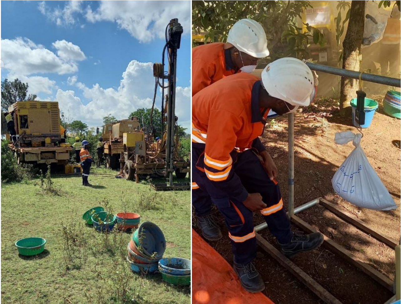
Figure 6: preparing RAB drilling pad on left and field assistants weighing clay samples (right) in preparation for dispatch to laboratory for testing in Perth.
