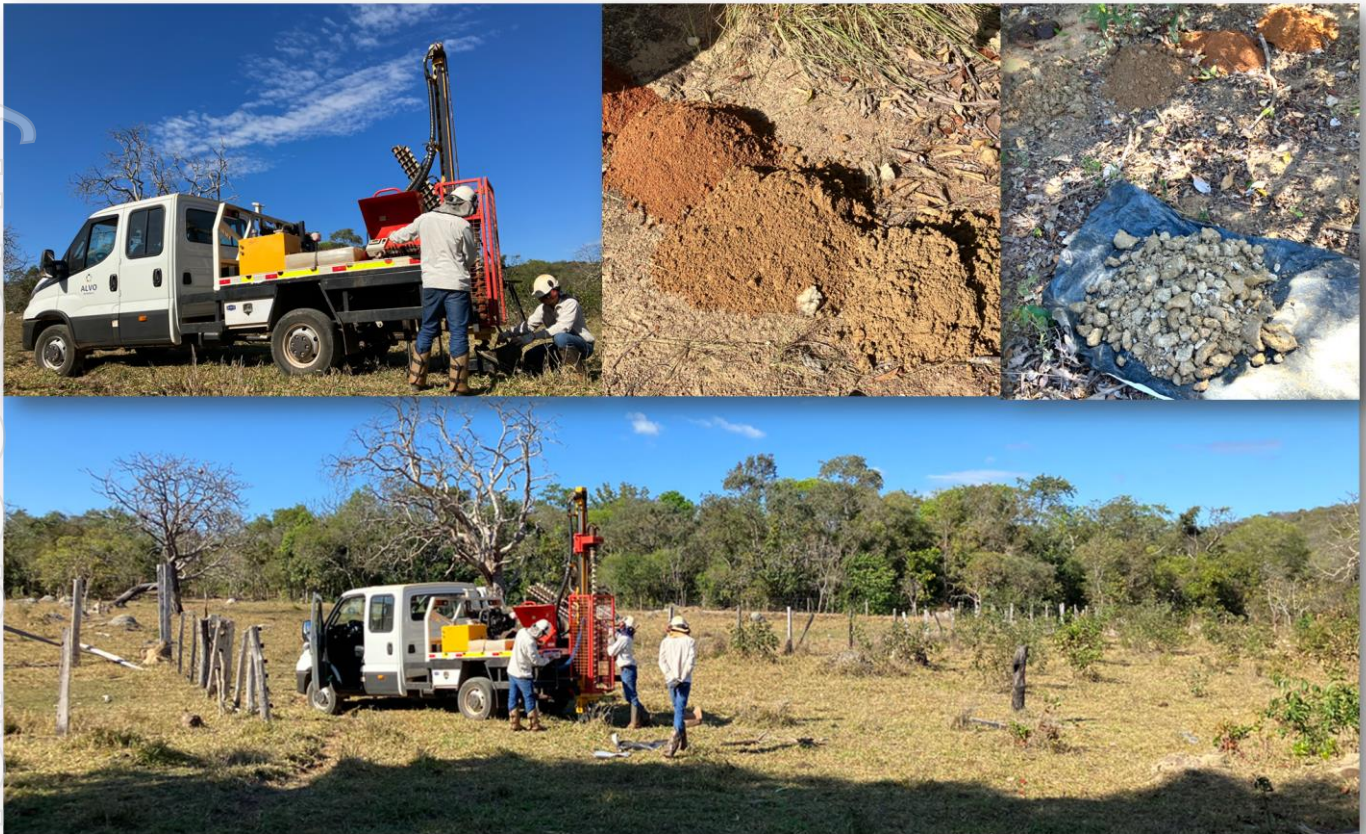
Figure 1 Alvo's auger rig drilling at Bluebush REE Project. Note the piles of samples representing saprolite intercepted in the hole (each pile represents a metre of advance).
