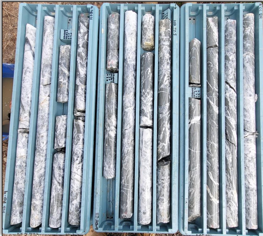
Figure 5: Extensive quartz-sulphide breccia zone in ERN005 from 73.9m to 84.4m.
