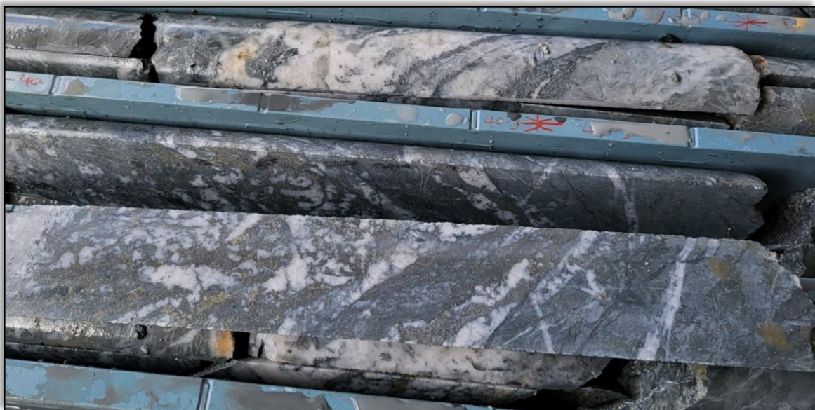
Figure 3: ERN0001 from 39m with laminated quartz-sulphide vein and brecciated sulphidic sandstone.
