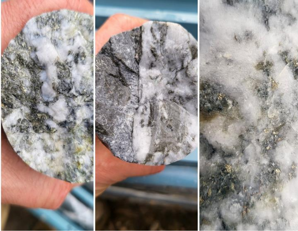
Figure 4: Core breaks from holes 3 & 4 highlighting the strongly disseminated sulphides including Arsenopyrite, Pyrite and Chalcopyrite sulphides.
