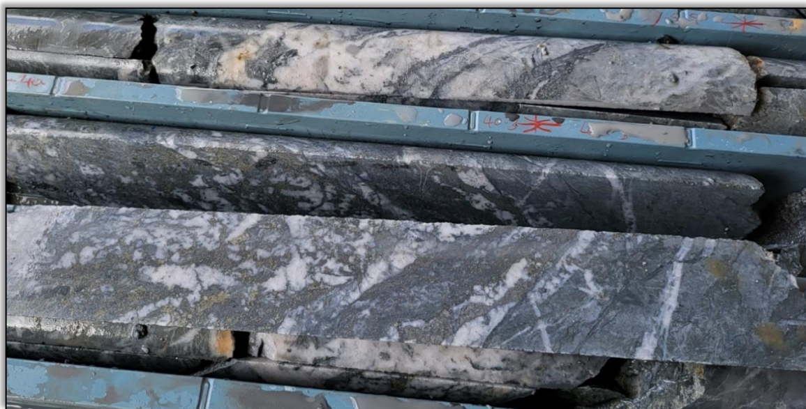
Figure 3: ERN001 from 39m with laminated quartz-sulphide vein and brecciated sulphidic sandstone.
