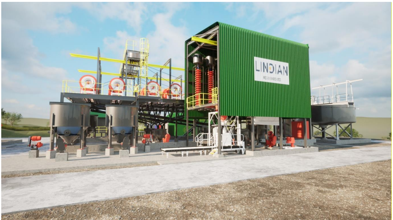
Image 4: Side view of the recovery circuit and concentrate filter press and packing shed and tails thickener (far right).
