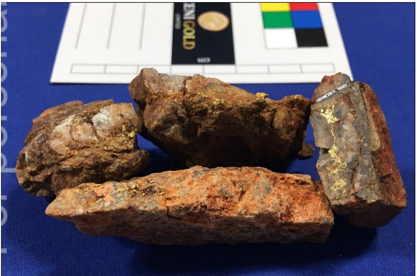
Figure 2 Specimen EV-4, gold taken from outcrop within the Christmas Gift anomaly (14UF010B). The peak assay was 18,207g/t Au.
