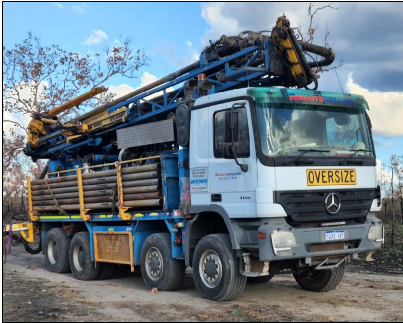
Photograph 1. RDS's RC drill rig arriving at the Enterprise Prospect at the Bynoe Lithium Project.
