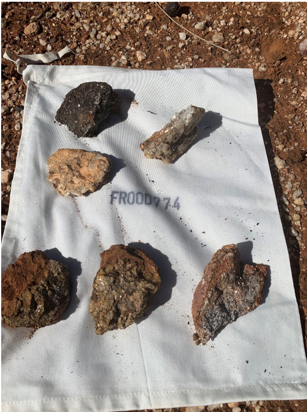
Figure 6: The Alexandra Bore/Breakaway Dam project area with muscovite bearing pegmatite sample, taken from the outcropping pegmatite in the previous image (Figure 5).
