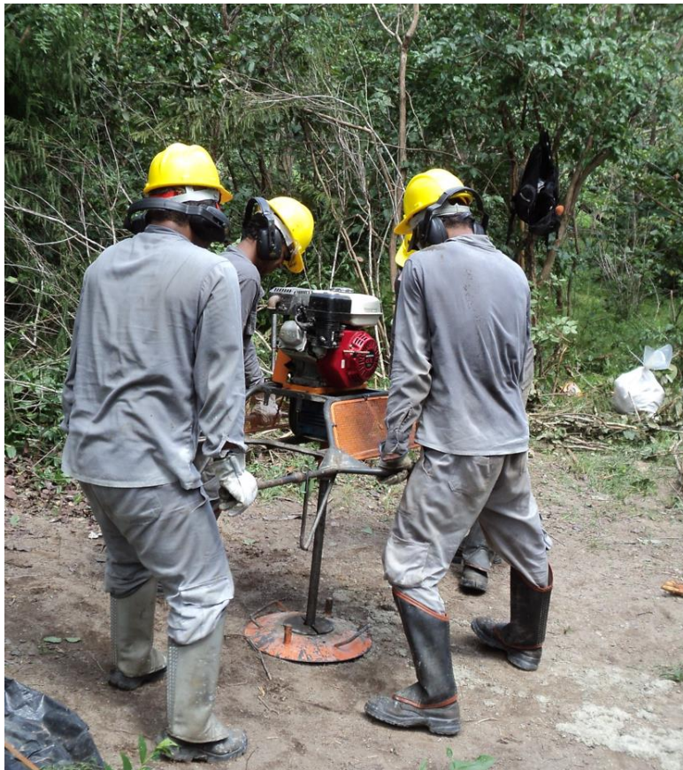
Figure 2: Photos from Mata Azul - Bluebush Exploration. Top left is an excavated pit with sampling intervals marked on left wall. Top right is measuring the thickness of an alluvial bank prior to sampling and the lower photo shows the handheld auger drilling.
