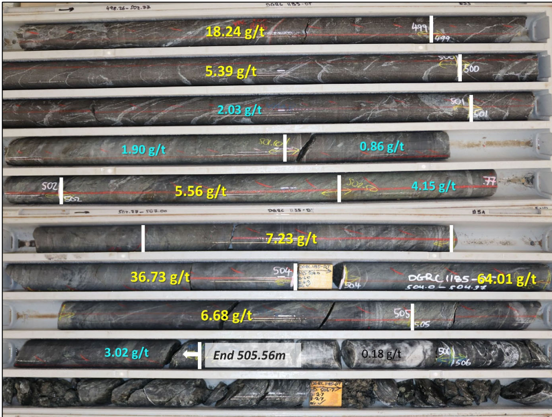
Figure 5b: Drill-core photos of DGRC1185-DT intercepting Never Never mineralisation from 488.16m downhole.
