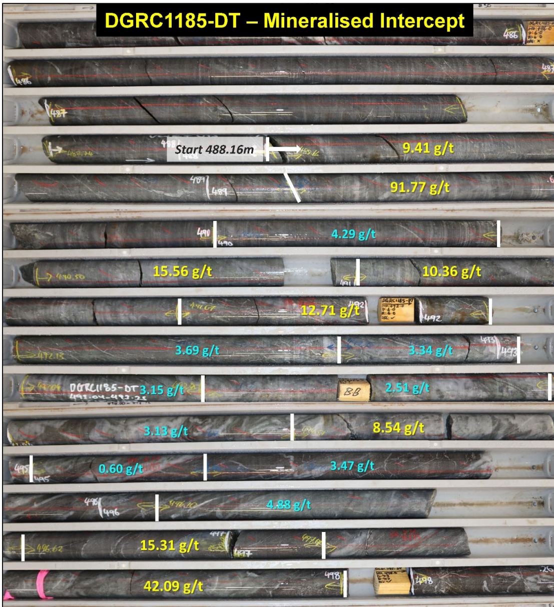
Figure 5a: Drill-core photos of DGRC1185-DT intercepting Never Never mineralisation from 488.16m downhole.
