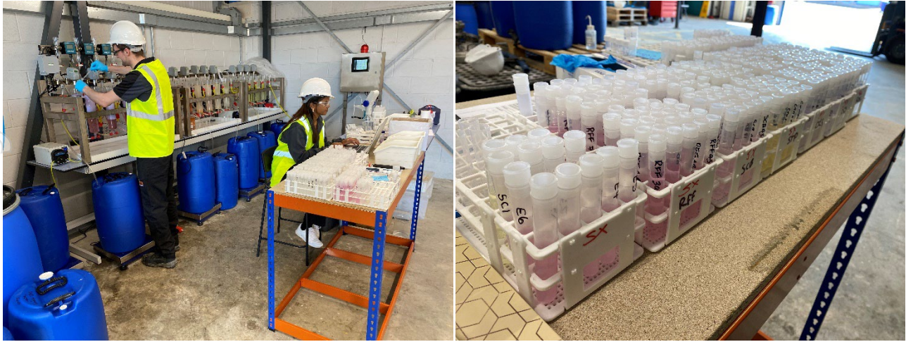
Figure 4: Pilot plant activities progressing in parallel, with solution samples analysed to finalise parameters for Demonstration Plant SX circuit commissioning and optimisation.
