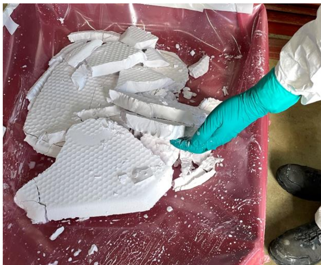
Figure 2: Final Mixed Rare Earth Carbonate (MREC) product produced from Pilot Hydromet Plant
