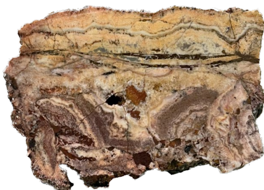
Figure 8 and Figure 9: 7250 - Colloform-crustiform quartz-chalcedony-adularia vein and quartz-hematite-adularia cockade breccia. No sulphides observed. 7255 - Crustiform-colloform quartz-chalcedony-adularia vein with quartz after bladed calcite and possible ginguro bands.
