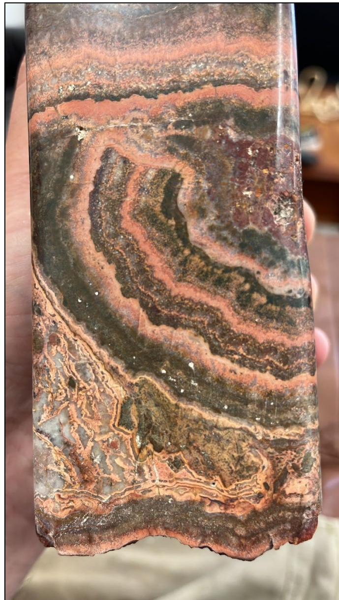
Figure 12: 7344 – Crustiform-colloform chalcedony-quartz-adularia-hematite vein. No sulphides observed.
