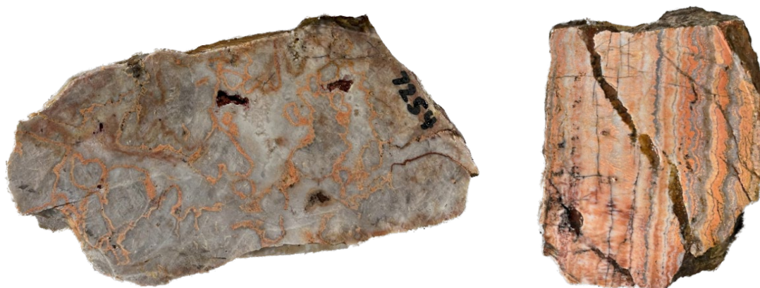
Figure 1: Rock chip samples taken from the newly discovered veins at the Breccia Sinter Prospect. 7254 – Chalcedony-quartz-adularia cockade breccia. 7257 - Crustiform-colloform banded chalcedony-quartz-adularia and quartz after bladed calcite vein. No sulphides observed. Note Cautionary statement about visible observations on Page 2.
