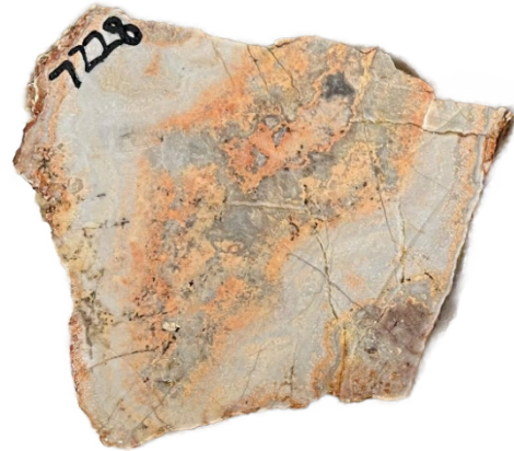
Figure 6 and Figure 7: 7247 - Chalcedony-quartz-adularia cockade breccia with possible ginguro banding. 7228 - Colloform-crustiform chalcedony-quartz-adularia vein. No sulphides observed.
