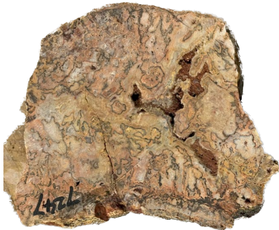
Figure 6 and Figure 7: 7247 - Chalcedony-quartz-adularia cockade breccia with possible ginguro banding. 7228 - Colloform-crustiform chalcedony-quartz-adularia vein. No sulphides observed.
