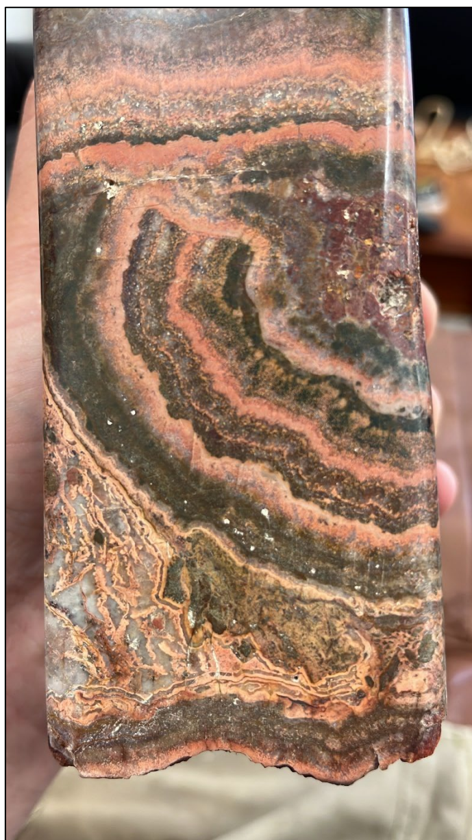
Figure 12: 7344 – Crustiform-colloform chalcedony-quartz-adularia-hematite vein. No sulphides observed.
