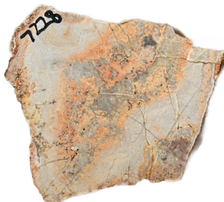
Figure 6 and Figure 7: 7247 - Chalcedony-quartz-adularia cockade breccia with possible ginguro banding. 7228 - Colloform-crustiform chalcedony-quartz-adularia vein. No sulphides observed.
