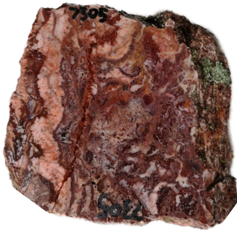
Figure 4 and Figure 5: 7305 – Custiform-colloform quartz-adularia vein clasts within quartz-hematite breccia. No sulphides observed. 7299 – Crustiform quartz-chalcedony vein with quartz after calcite. No sulphides observed.
