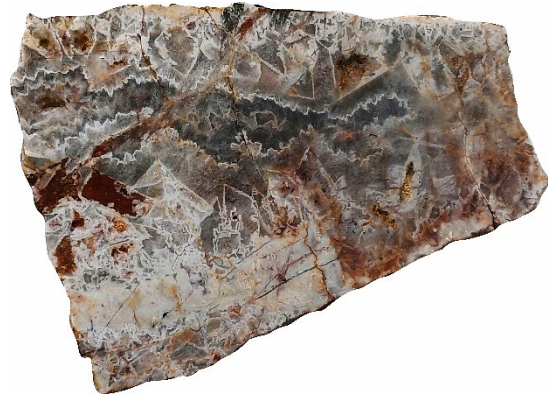
Figure 4 and Figure 5: 7305 – Custiform-colloform quartz-adularia vein clasts within quartz-hematite breccia. No sulphides observed. 7299 – Crustiform quartz-chalcedony vein with quartz after calcite. No sulphides observed.
