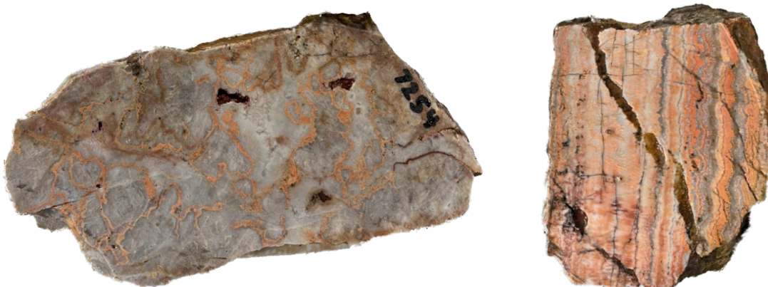
Figure 1: Rock chip samples taken from the newly discovered veins at the Breccia Sinter Prospect. 7254 – Chalcedony-quartz-adularia cockade breccia. 7257 - Crustiform-colloform banded chalcedony-quartz-adularia and quartz after bladed calcite vein. No sulphides observed. Note Cautionary statement about visible observations on Page 2.
