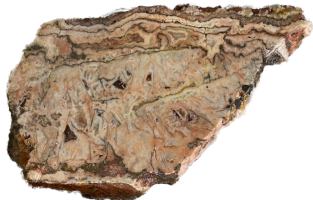
Figure 8 and Figure 9: 7250 - Colloform-crustiform quartz-chalcedony-adularia vein and quartz-hematite-adularia cockade breccia. No sulphides observed. 7255 - Crustiform-colloform quartz-chalcedony-adularia vein with quartz after bladed calcite and possible ginguro bands.
