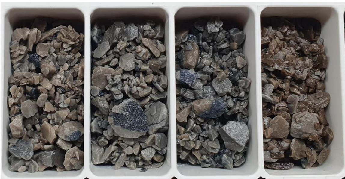
Figure 1: Example of RC chips from drill hole SR23-03 displaying chalcocite (gun metal grey) breccia and veins within dolomite from approximately 79.2 – 85.3m downhole. This interval assayed 3.2% Cu.
