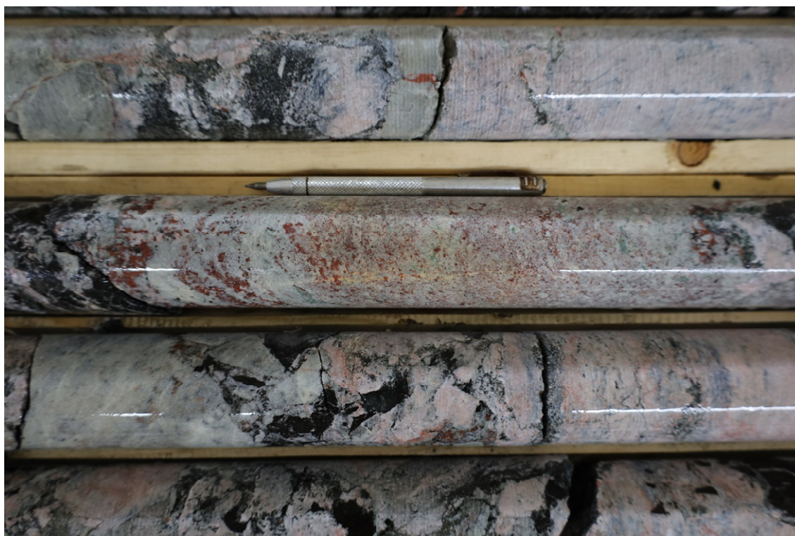
Figure 3: Diamond drill core (NQ, approximately 4.8 cm diameter) containing REE mineralisation (red coloured disseminations) within ferrocarnatite/calciocarbonatite host rock. Hole POM-23-01, Box 15, 91.1 – 95.5 metres downhole depth.
