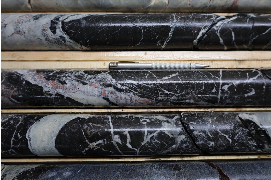
Figure 4: Diamond drill core (NQ, approximately 4.8 cm diameter) containing REE mineralisation (red coloured disseminations) within silicocarbonatite host rock. Hole POM-23-01, Box 3, 39.0 – 43.5 metres downhole depth.
