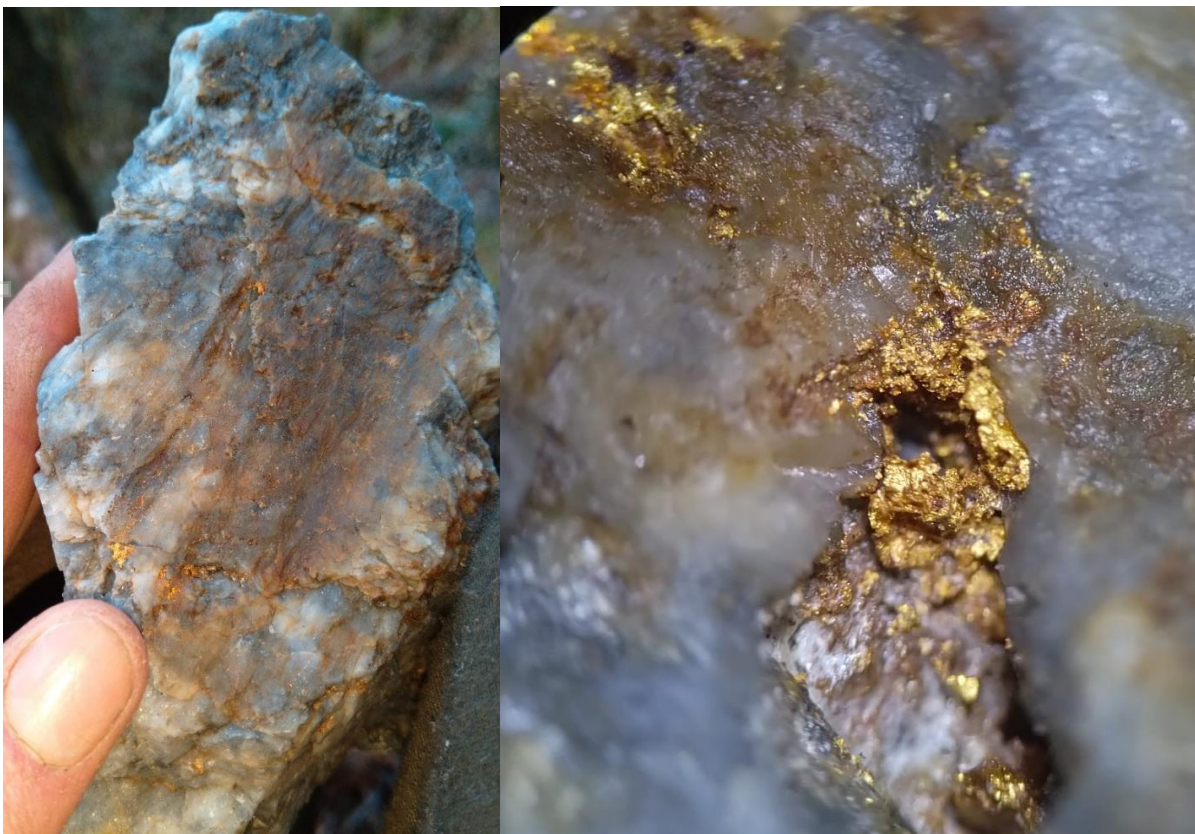
Figure 5. United Victory Reef float sample that assayed 205g/t Au
