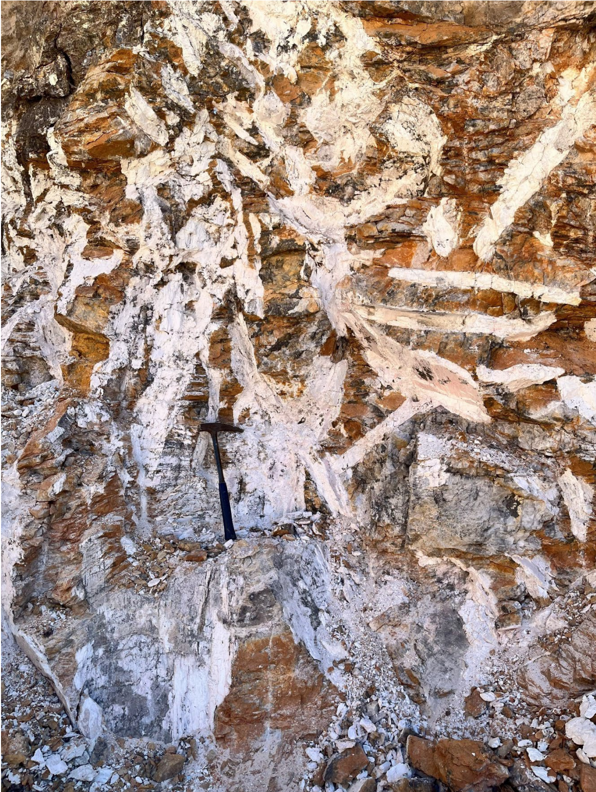
Figure 2: Large white weathered spodumene crystals within Jaguar artisanal workings-G Pick for scale
