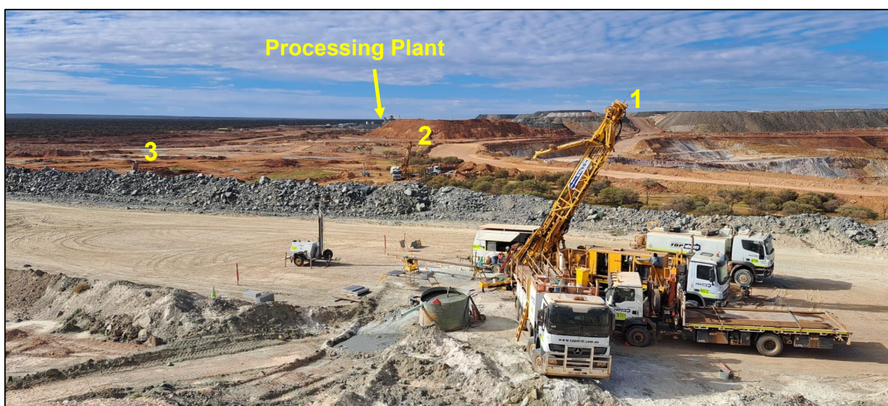
Figure 1: Three drill rigs (two diamond rigs – #1 & #2 and 1 RC rig – #3) drilling out the high-grade Never Never Gold Deposit with the 2.5Mtpa Dalgarranga Process Plant in the background.
