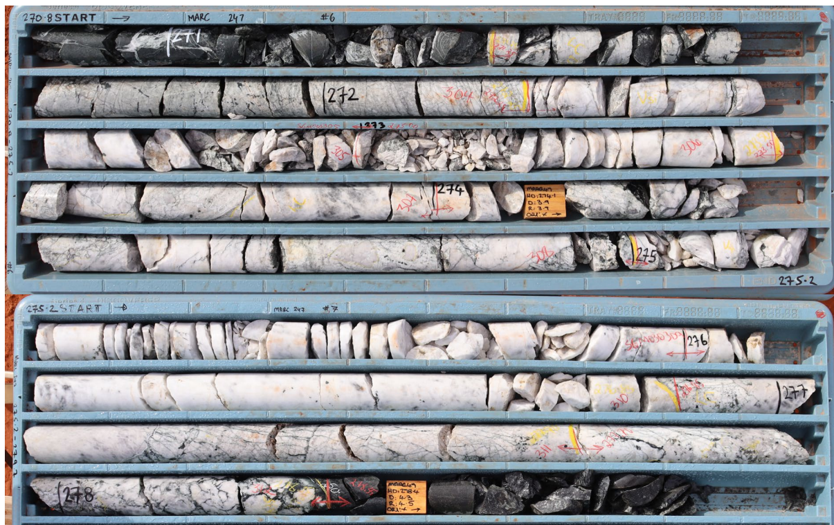
Figure 1 – MARC247 drill core showing pegmatite from 271.25m to 278.35m (awaiting assays).
