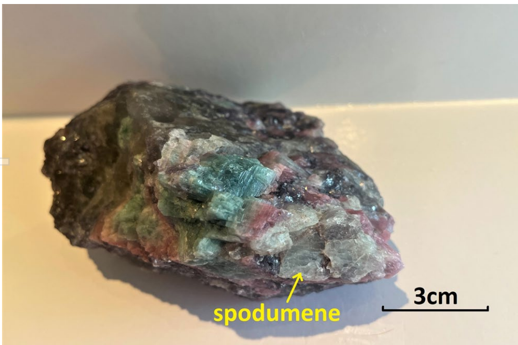
Figure 4: Specimen of spodumene-bearing rock from Muvero East. Rock comprised of approximately 50% lepidolite, 35% quartz, 10% elbaite (pink and green) and 5% spodumene.
