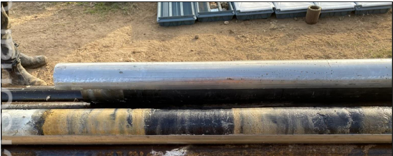
Figure 4: Cobalt in manganese oxide horizon in hole Codd001 returning 1.05m @ 0.26% cobalt, including 0.25m @ 0.83% cobalt at the base of a 12.45m interval of sediments with heavy minerals sands returning 3.28% TiO 2 from 7.1m depth.
