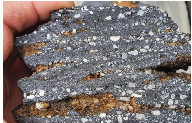
Figure 2: surface sample of cobalt enriched, manganese replacement rock returning 1.19% cobalt, 0.24% nickel and 13.4% manganese.
