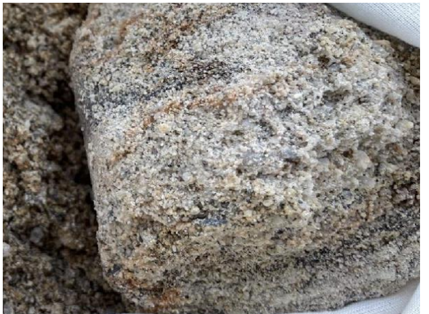
Figure 3: Example of unconsolidated sediment material hosting heavy mineral sands from hole CODD02, returning 5.9% TiO 2 from 7 to 7.5m depth interval.
