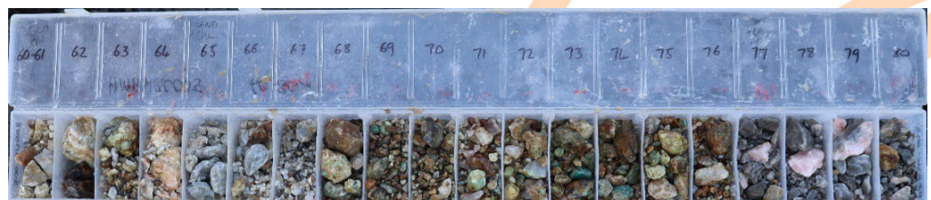
Figure 1. HMHW005 60-80m showing copper oxide mineralisation. 9m at 1.51% Cu and 0.18% TREYO from 67m
