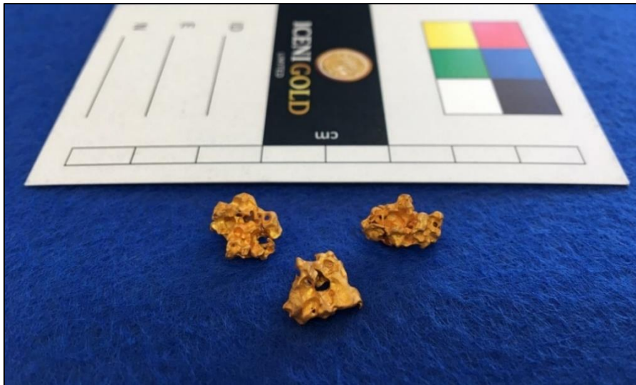
Figure 5 Salt lake gold nuggets recovered from Guyer North with a gold fineness of ~97.5% (by pXRF)*.
