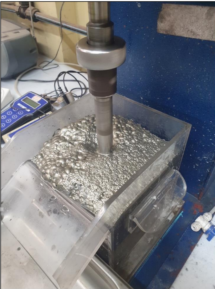
Figure 17: MOB02 flotation test in progress
