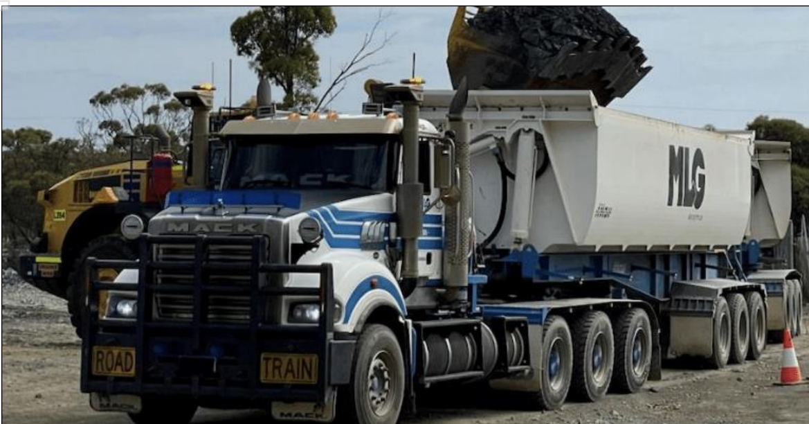
Figure 20: Typical road-train loading and haulage arrangement
