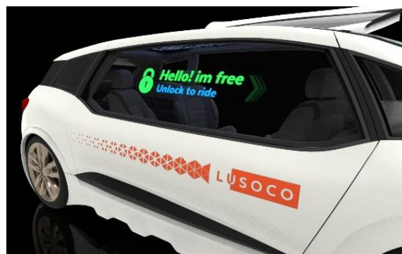
Artist's impression of automotive application demonstrating how different coloured invisible fluorescent inks can be selectively activated using different light wavelengths.
