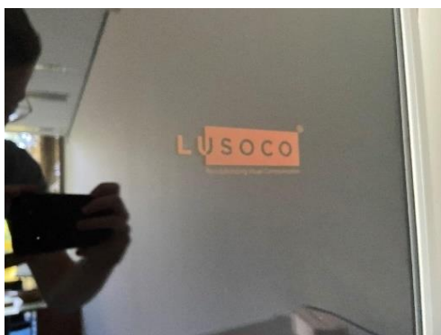
Pattern printed in invisible fluorescent ink in background of clear glass panel.
