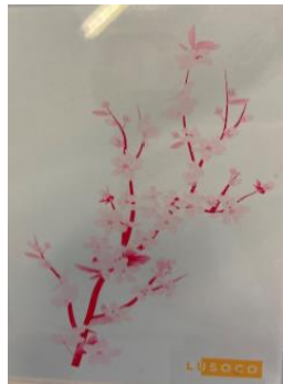
Pattern printed into glass using visible fluorescent inks
