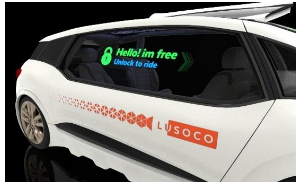
Artist's impression of automotive application demonstrating how different coloured invisible fluorescent inks can be selectively activated using different light wavelengths.
