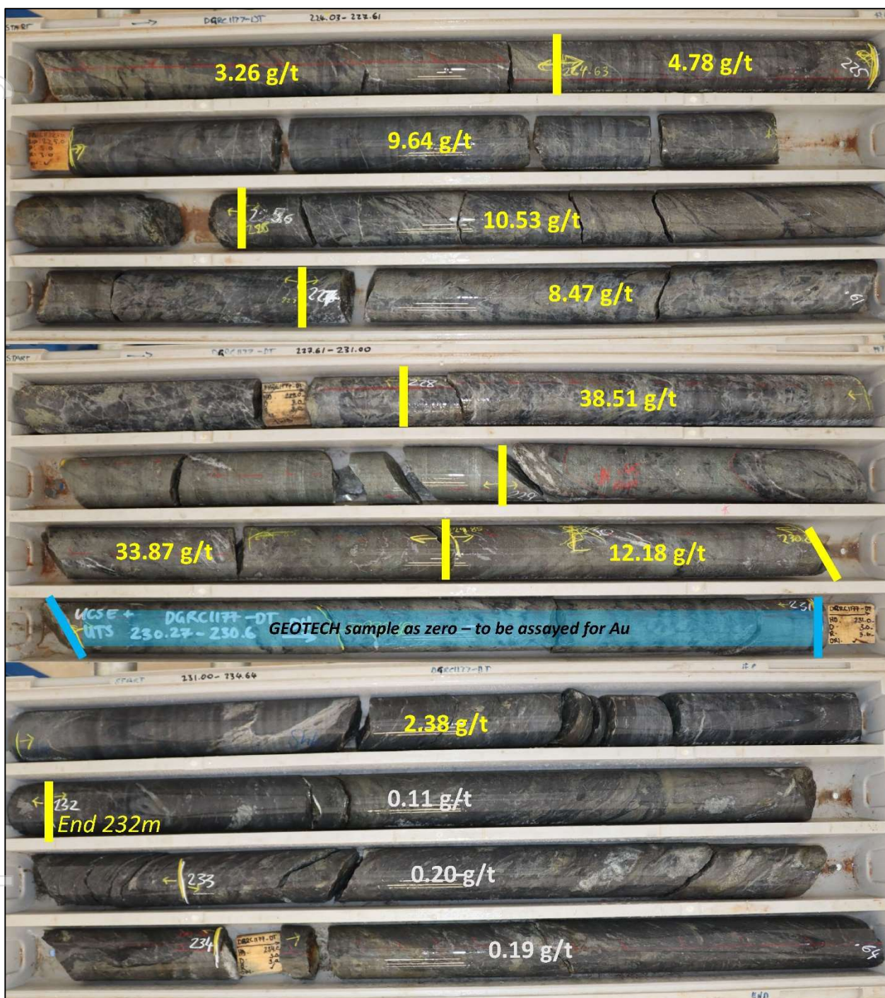
Figure 6: Photographs of drill-core from DGRC1177-DT (15.7m @ 13.51g/t Au) from the Never Never Gold Deposit. Silica “flooding” and sericite/biotite alteration is evident throughout the consistent high-grade mineralisation. Note: two intervals labelled as “GEOTECH” are given a value of 0.00g/t Au for the purposes of calculating the total intercept.
