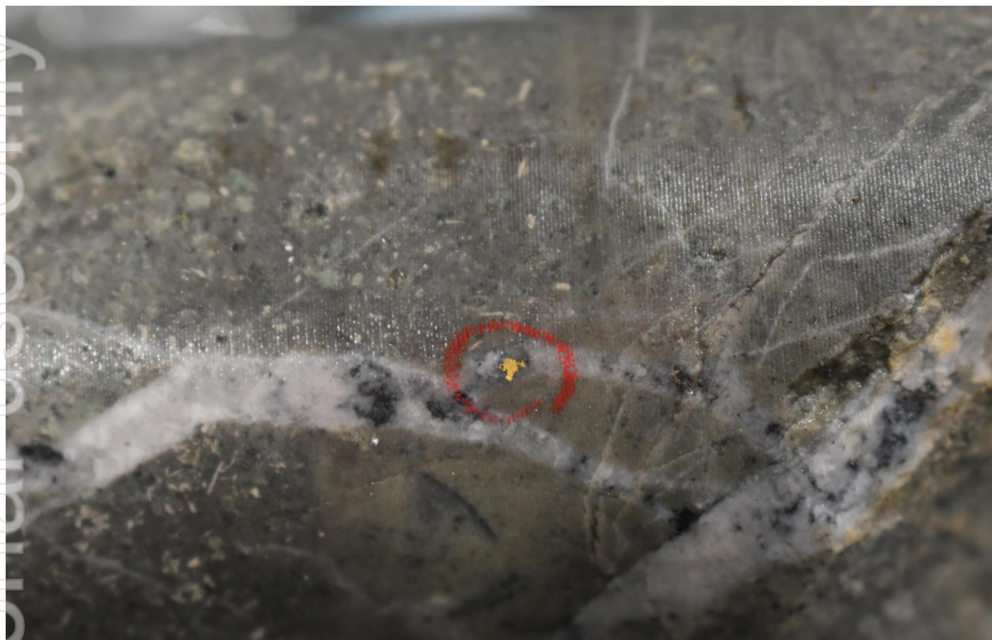
Photo 3: SDDSC064 between 890.2-890.7 m showing visible gold within a quartz carbonate vein stockwork hosted by albitised and sericitized dioritic dyke. Minor fuchsite (lime green) alteration in dyke. Field of view 30mm.
