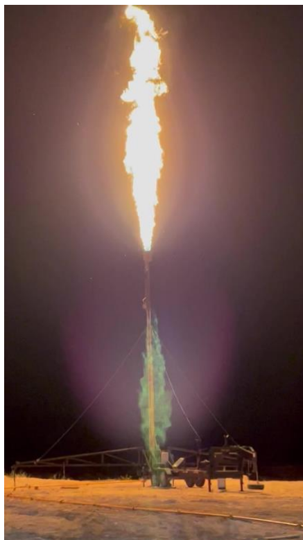
Photo: Flaring gas from Presidio 52#1 well.
