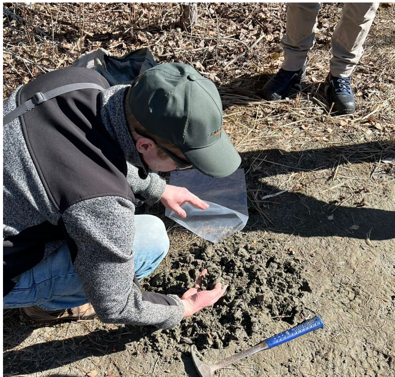
Figure 4. Sampling Korsnäs TSF for remnant rare earth oxides. Samples are currently being analysed at ALS Outokumpu Finland.
