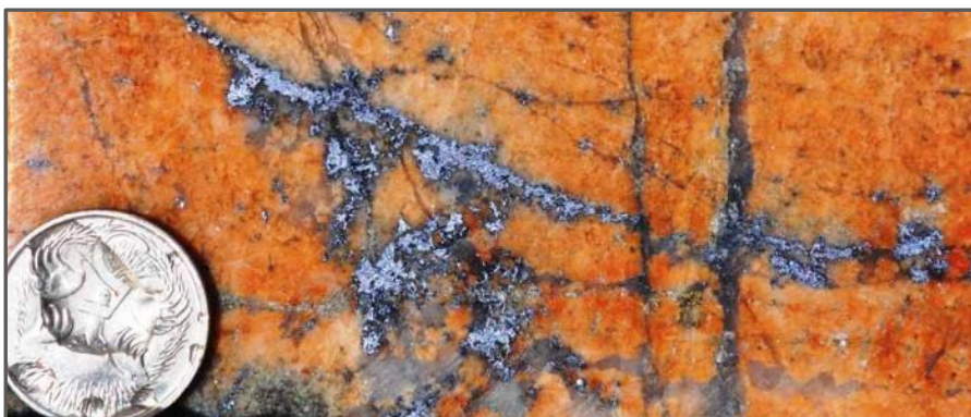
Image 1: Anthony Mo Deposit - Example of molybdenum mineralisation in oxide/transition zone
