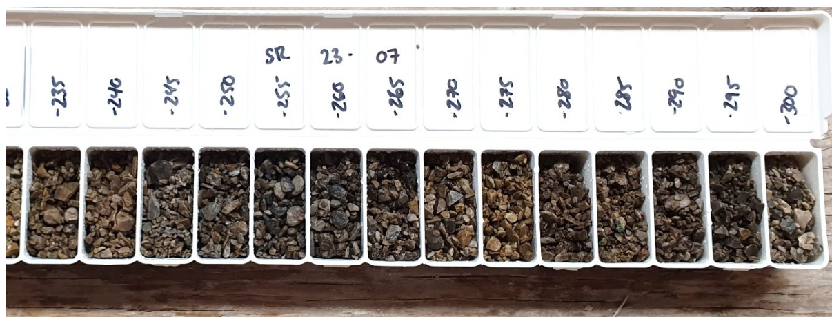
Figure 6: RC drilling chips from SR23-07 between approximately 72 – 91m (235 – 300ft) downhole. Chalcocite (copper sulphide) can be seen as dark grey chips.
