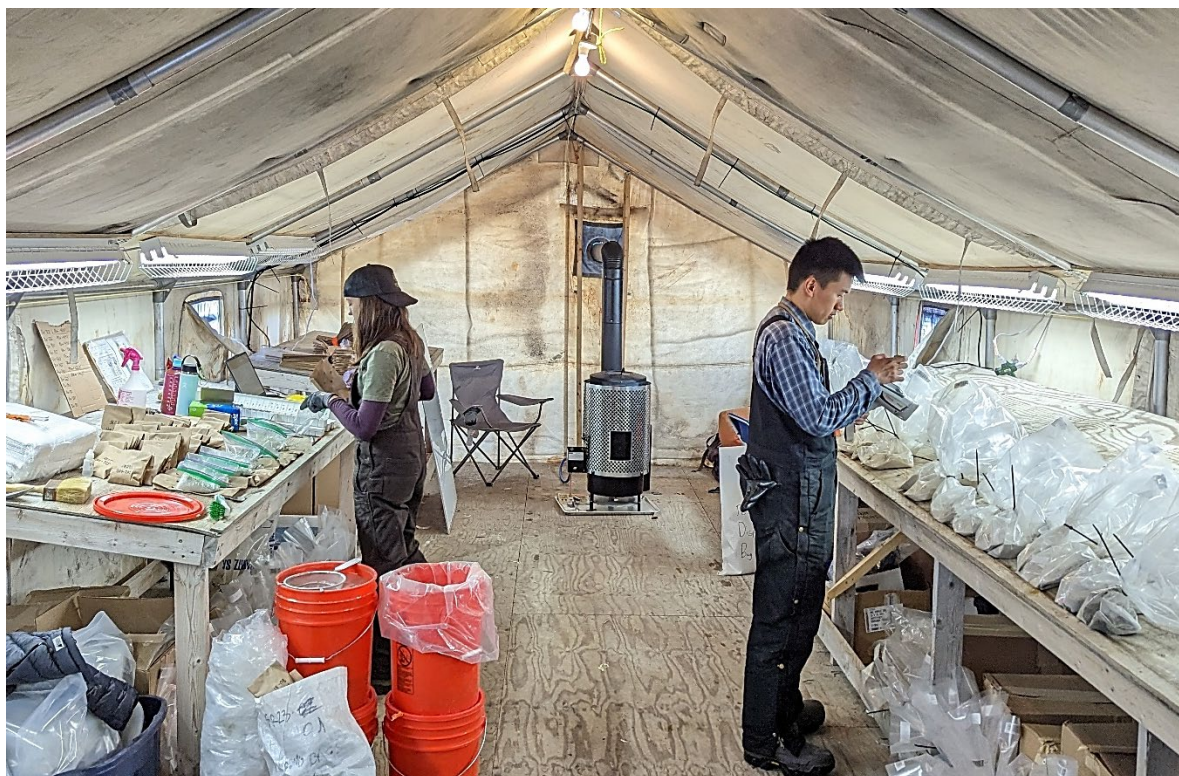
Figure 1: RC samples being analysed with portable XRF and prepared for shipment to the laboratory, Storm Copper Project.
