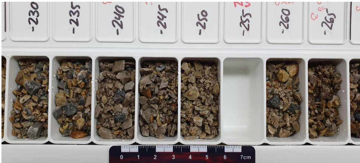
Figure 7: RC drilling chips from SR23-08 between approximately 70 – 81m (230 – 265ft) downhole. Chalcocite (copper sulphide) can be seen as dark gray chips.
