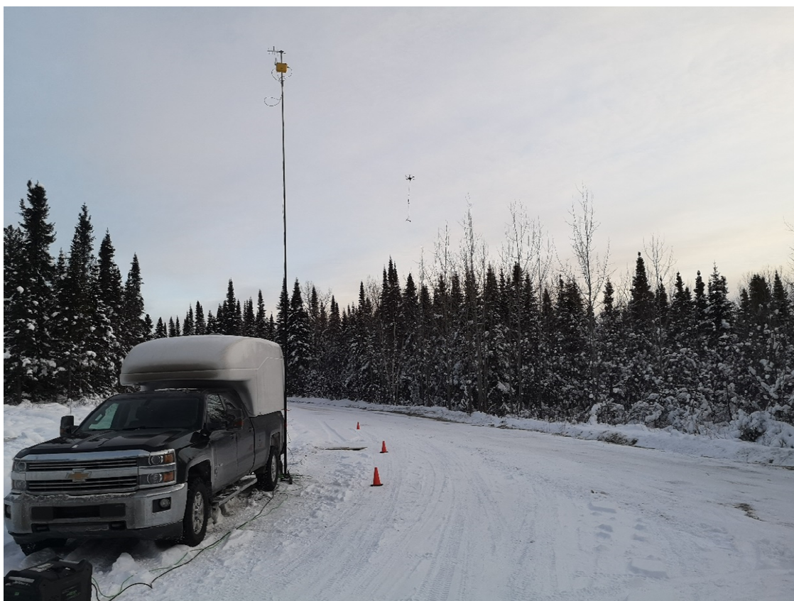
Figure 1: Drone magnetic survey operations at the Pomme REE-Nb project in early April 2023 (courtesy Vision 4K).
