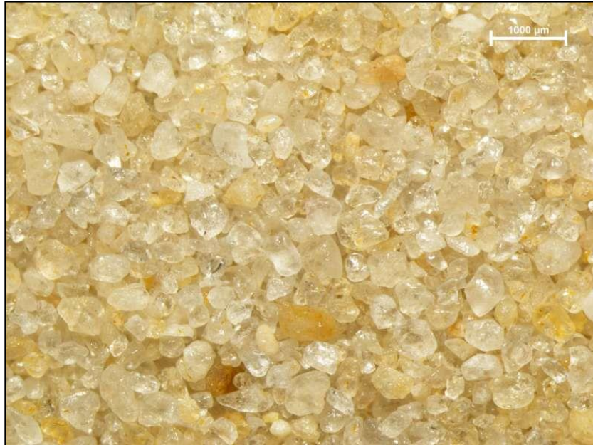
Photomicrograph of VRX 'AFS55' foundry sand product, showing sub-rounded quartz grains
