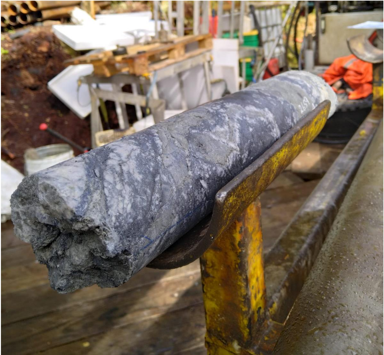
Figure 1. Stibnite (black) cemented host rock breccia from ACDDH004 at 131.4 to 131.8m that assayed 6.7g/t Au, 20.9% Sb for 56.0g/t AuEq.
