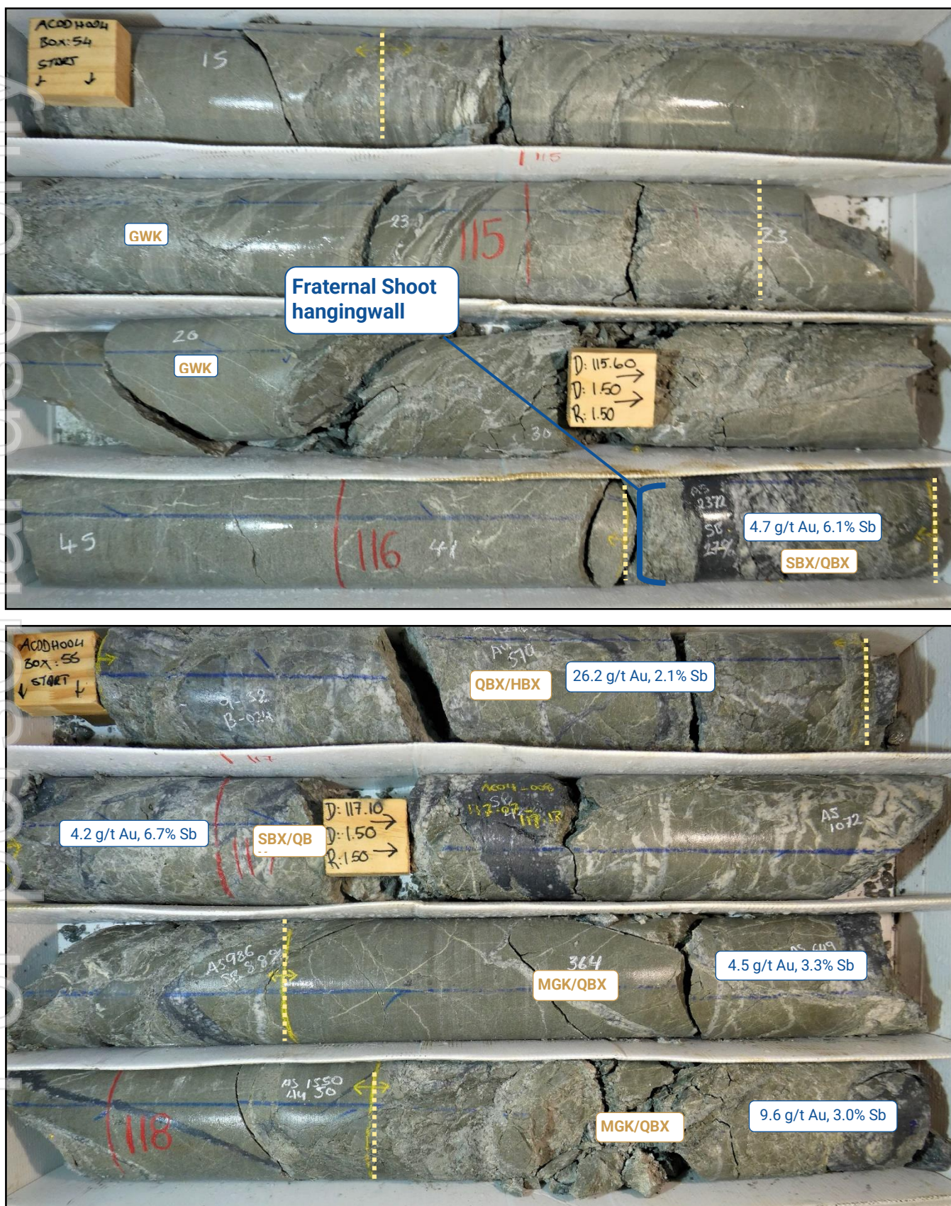
Figure 5a. Fraternal Shoot intersected in AXDDH004 116.2m – 118.4m. (SBX - stibnite cemented breccia, QBX – quartz breccia, HBX – host rock breccia, MGK – silicified disseminated arsenopyrite mineralised greywacke, MAR - silicified disseminated arsenopyrite mineralised argillite).
