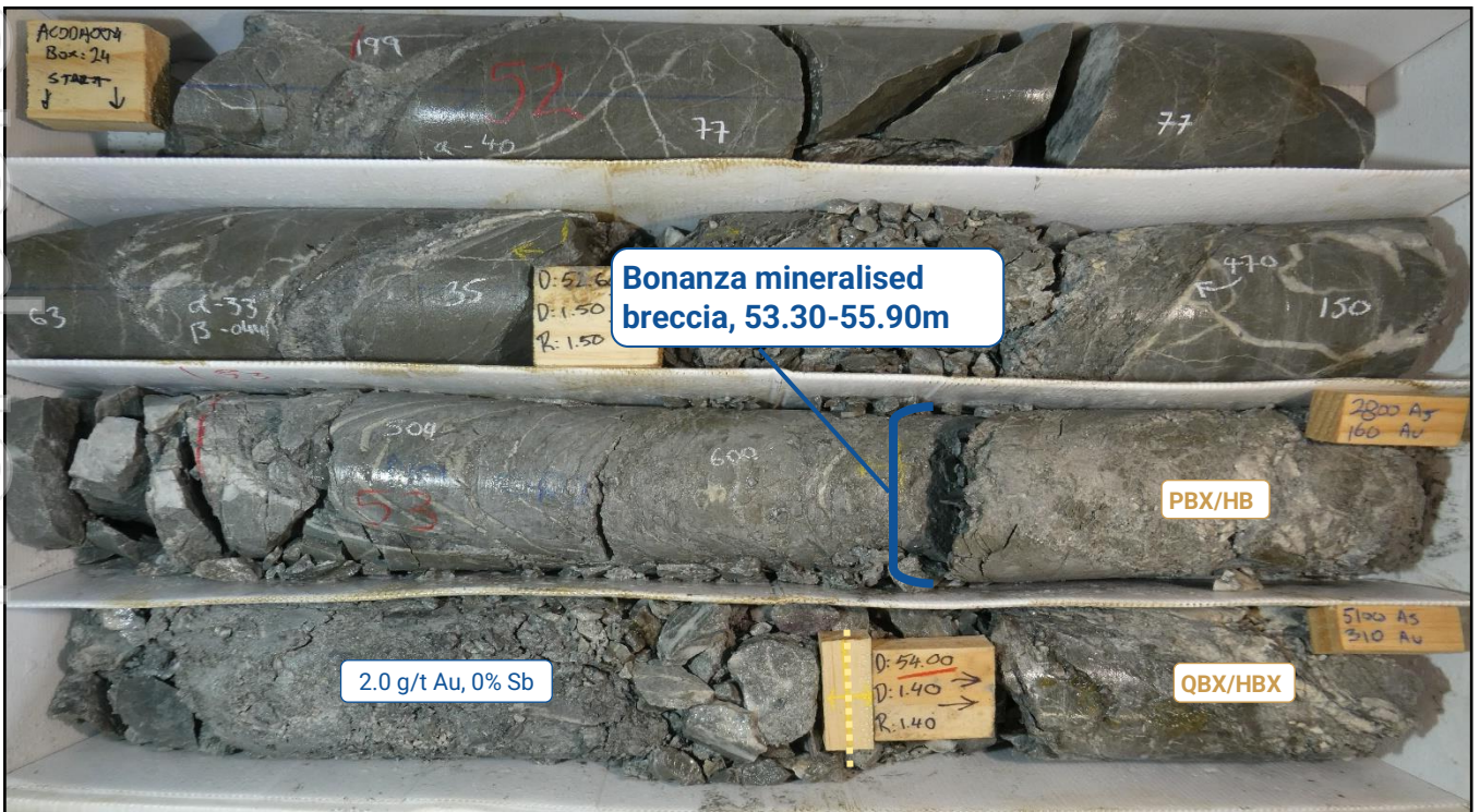
Figure 7a. Bonanza Shoot intersected in AXDDH004 53.3m – 54.2m (SBX - stibnite cemented breccia, QBX – quartz breccia, HBX – host rock breccia, MGK – silicified disseminated arsenopyrite mineralised greywacke, MAR - silicified disseminated arsenopyrite mineralised argillite).
