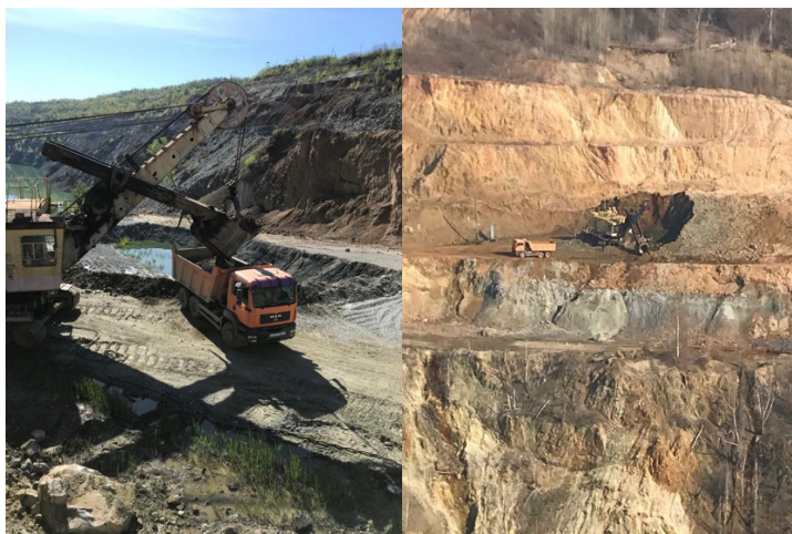
Figure 1 – Graphite Ore being Loaded and Hauled in the Zavalievsky Mine, April 2023
