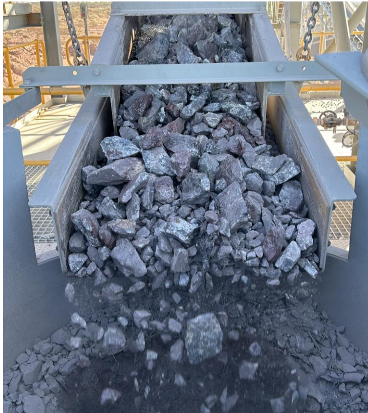
Figure 2 – Ore feeding into the secondary crusher at Abra (photo 3 May)
