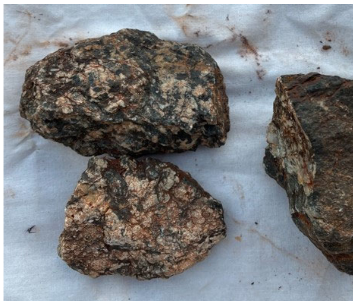
Photo 1: CGRC045–0.6g/t Au with elevated Ba(220ppm),Cr(245ppm),Mn(1,060ppm),P(1,000ppm)and Sr(577ppm)
