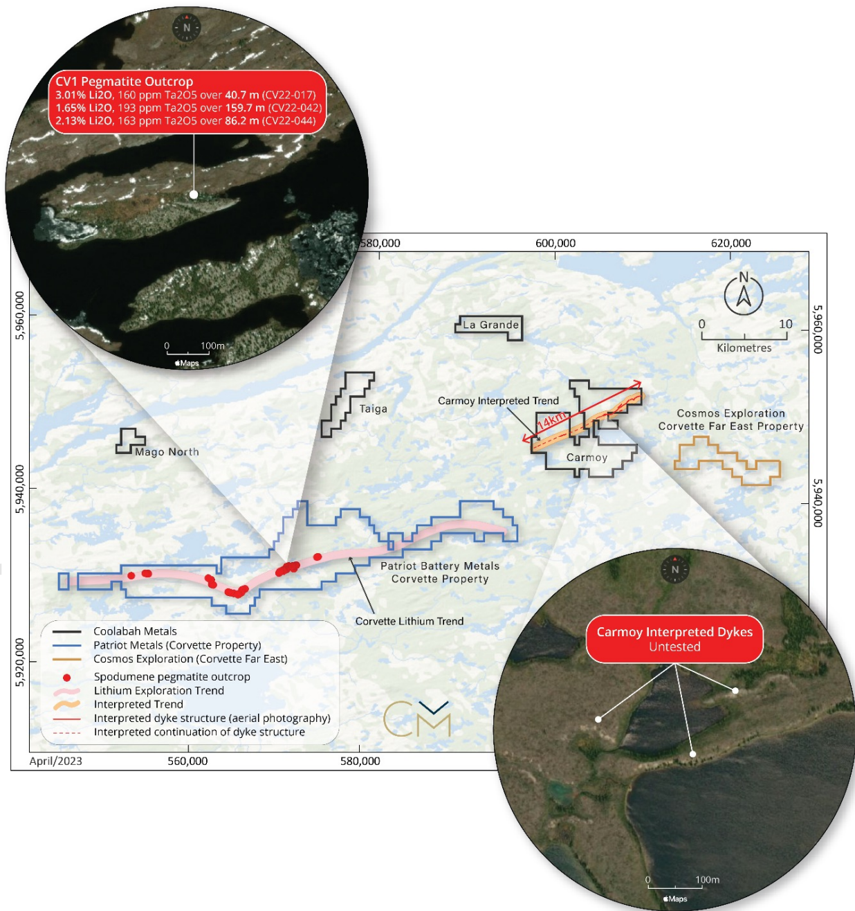
Figure 2: Hampden Project Claims Highlighting interpreted trends of untested dykes within the Carmoy property relative to Patriot's Corvette Lithium Trend
