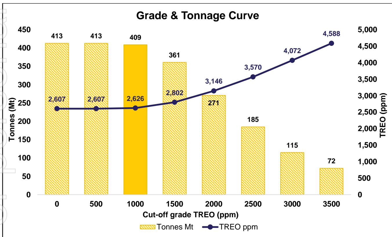
**Figure 7.** Grade Tonnage Curve Caldeira REE Project.
