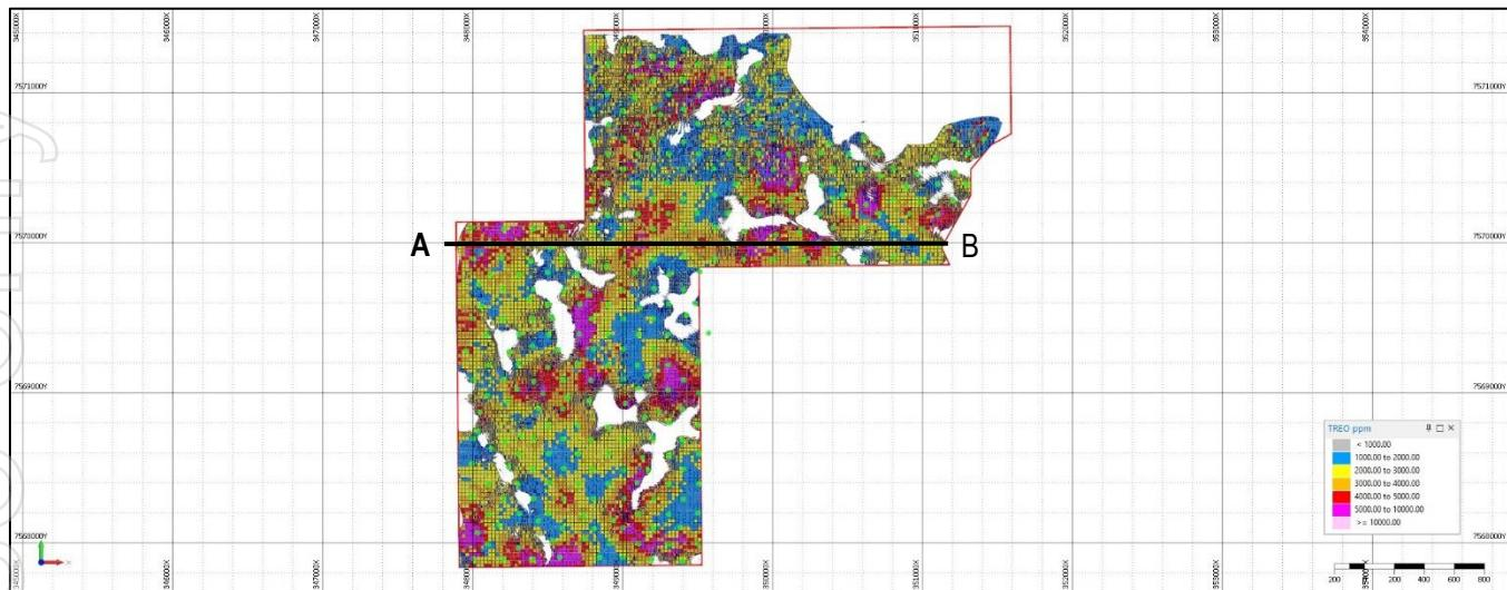
**Figure 6A.** Grade distribution plan (block model) Soberbo.
