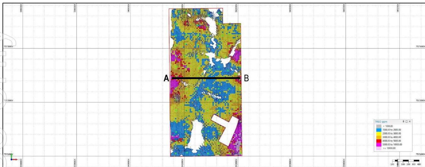
**Figure 5A.** Grade distribution plan (block model) Figueira
