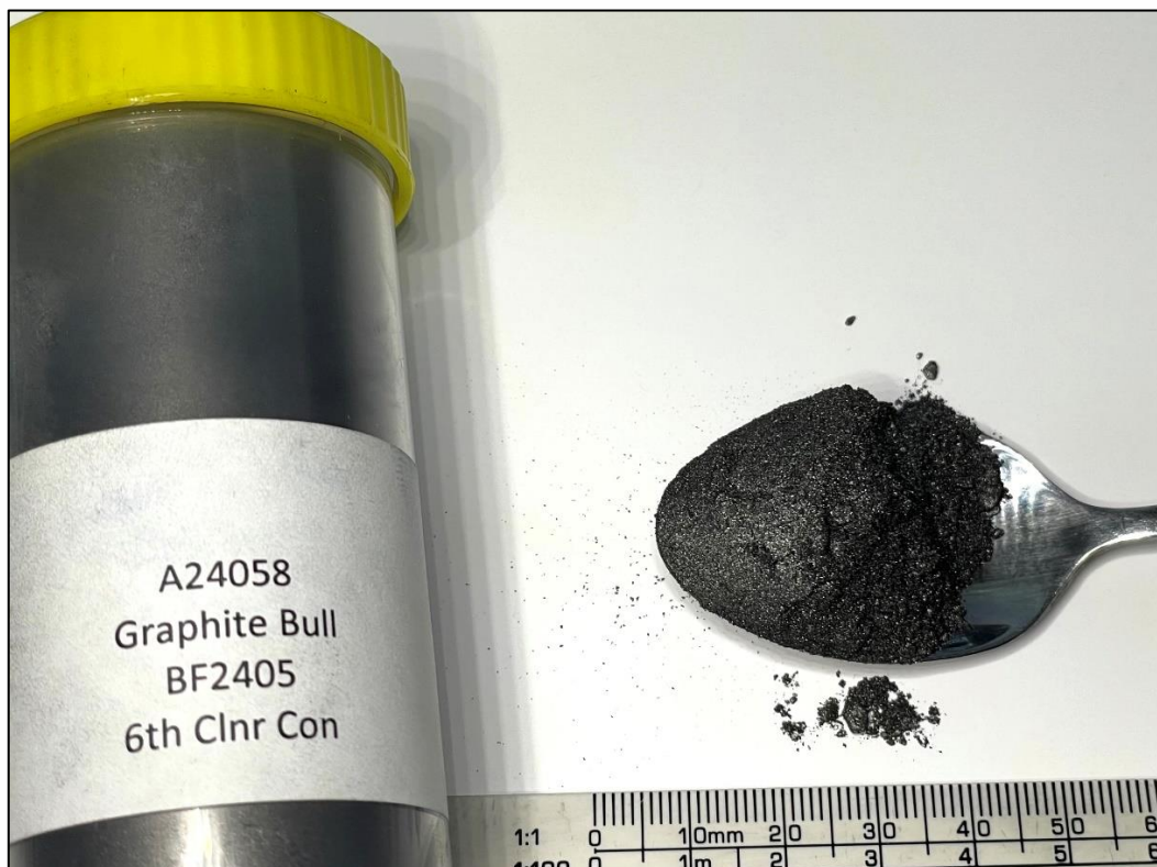
Figure 1: Graphite Bull graphite concentrate from recent flotation test work.
