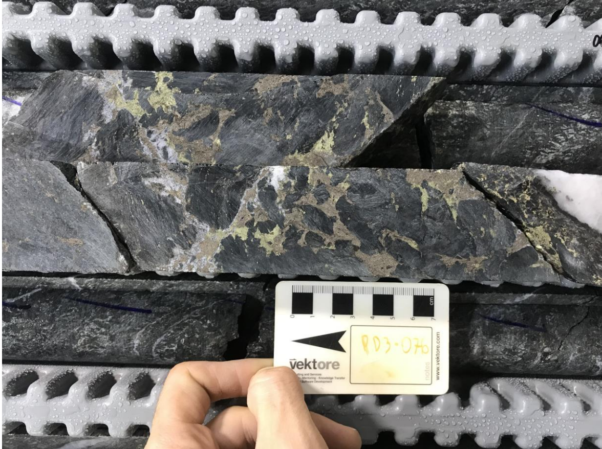
Figure 2: Core photo of PD3-076, depth of 438.7m with brecciated amphibolite disseminated/ semi-massive sulphides with chalcopyrite (gold colour) and Pyrrhotite (bronze colour)
