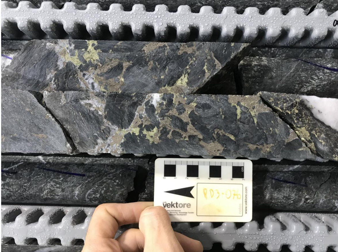
Figure 2: Core photo of PD3-076, depth of 438.7m with brecciated amphibolite disseminated/ semi-massive sulphides with chalcopyrite (gold colour) and Phyrrotite (bronze colour)
