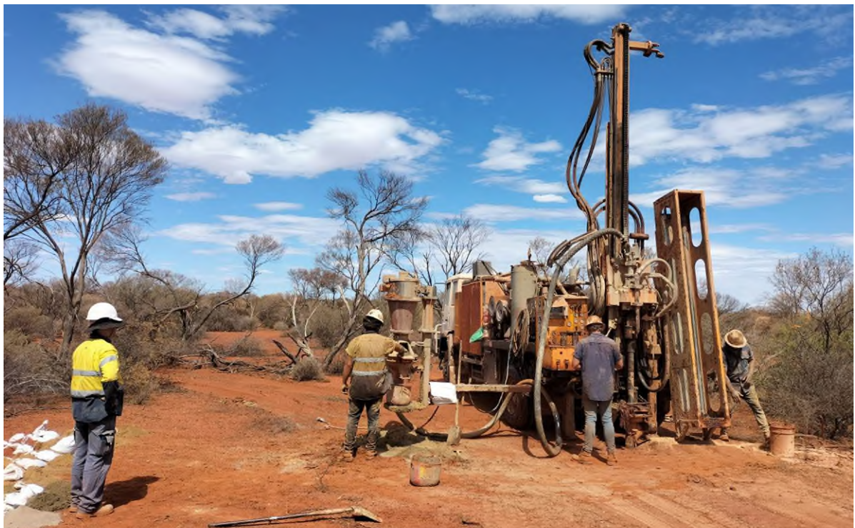
Figure 8: Aircore drilling underway at the Pt Kidman Prospect in January 2023.
