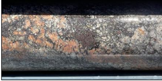
Figure 13. Photo showing an example of granite found in drill core from Central DD003.
