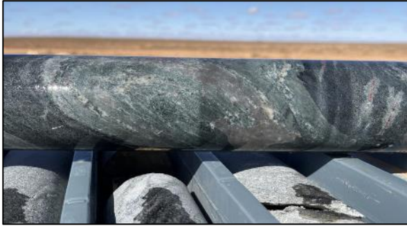
Figure 11. Initial first-pass observation of stage 2 hydrothermal alteration of host rocks. Initial observations indicate epidote-chlorite-sericite +/- actinolite and biotite alteration. Diamond HQ drill core Central_DD003.
