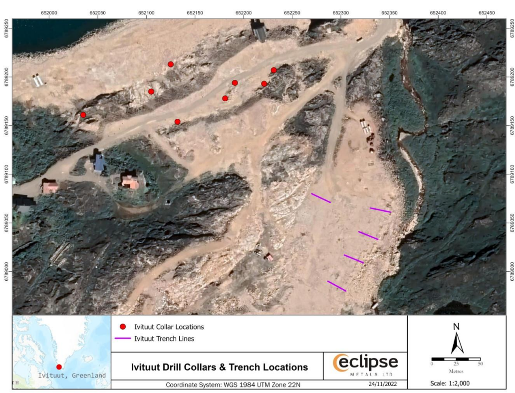
Figure 2: Ivigtût target area. Drill collars are marked with red dots. Bulk sample trenches are marked with purple lines.
