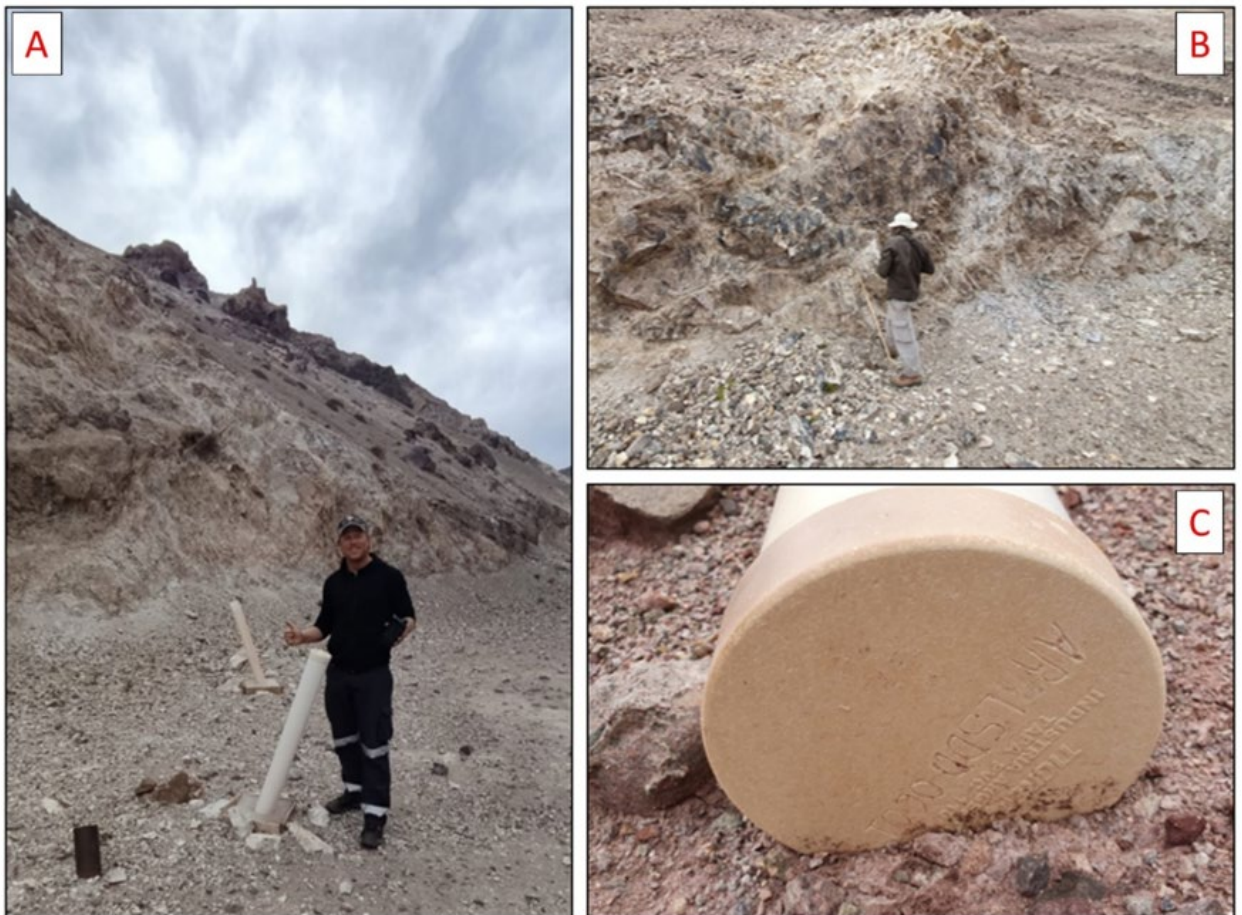
Figure 3: Position A - image showing collars of ARRLSDD00002, ARRLSDD00003 and T4D and an exposed, altered dacite outcrop; Position B – an intensely weathered dacite outcrop exhibiting intense and pervasive argillic alteration. Disseminated mineralisation was observed as oxidised sulphides throughout the rock outcrop and within veinlets Position C – photo shows cap on the ground at collar location for ARRLSDD00001.
